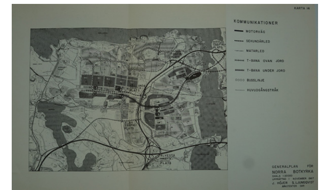
Figure 6: Plans for transport communication Northern Botkyrka (1967). 4 subway stations were constructed, and 2 bus lines were planned to connect people to the subway stations. (Source from Botkyrka Municipal Archive, Generalplan för Norra Botkyrka, 1967).
